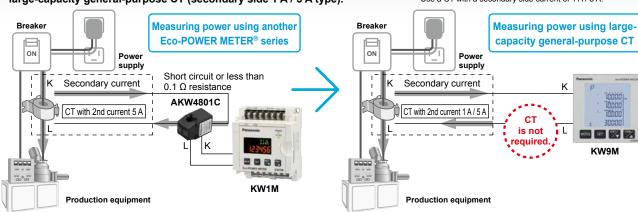
The measuring accuracy of the Eco-POWER METER® does not take the CT error into account. Other Eco-POWER METER® series (except AKW8115) need to use two CTs for measurement. KW9M is ready for direct input from only one CT, allowing higher accuracy measurements than with other Eco-POWER METER® series.
